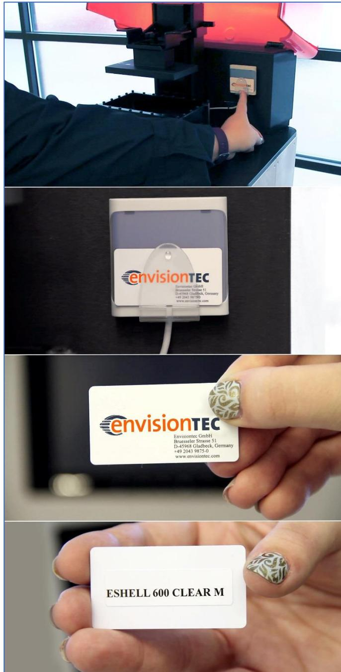
*EnvisionTEC resins come with an RFID material tag that conveys specific information to the 3D printer about the "Build Styles" to be used to optimally print a specific material. For example, not all materials should be printed at the same Z layer thickness.*
