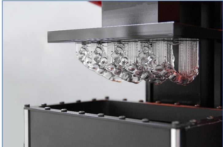
*These bite guards were printed in EnvisionTEC's clear E-Guard material nested together on a slight slant as a strategy to more accurately print this clear material.*
