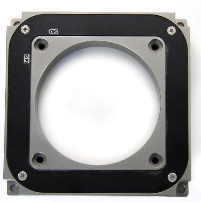
*This is photograph of the EnvisionTEC Enhanced Resolution Module. The projector shines through the center of the ERM, which moves the projector a half pixel in X and Y, to shift the second exposure in a sophisticated 3D anti-aliasing technique.*
